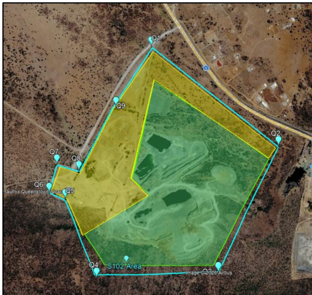
Figure 7: Satellite image of the mining area (blue polygon) to be rehabilitated upon closure. The mining and processing related areas (yellow) will revert to agricultural/residential use upon rehabilitation, and the quarry excavations (green) will be rendered safe and left as a landscape feature. (Image obtained from Google Earth)
