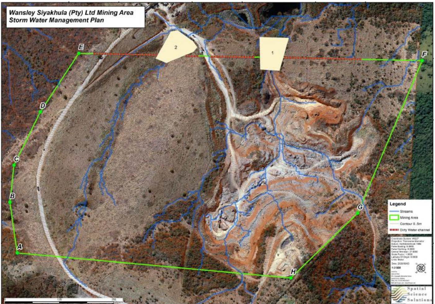
Figure 4: Image showing the drainage lines within the mining footprint (blue lines) as well as the proposed position of the stormwater dams (light yellow polygons) (image obtained from the SWMP).
