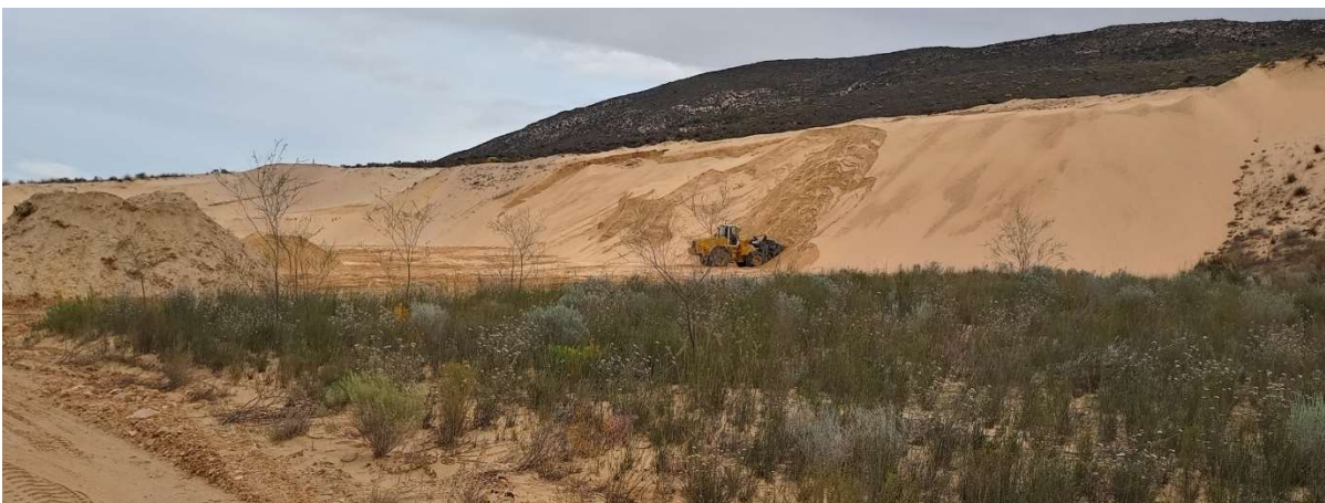
Photo 1: The current Zandberg mine operations with front-end-loader working on the sand face
