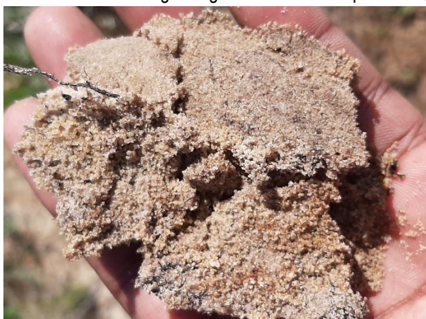
Photo 7: Soil sample extracted from the artificial wetland habitat. Note the low chroma orange mottles in the soil matrix.
