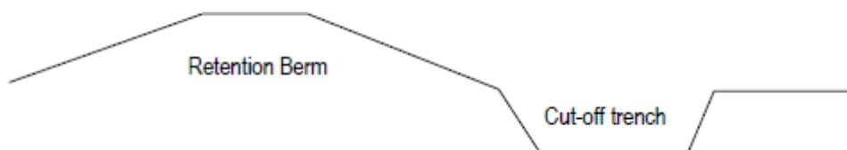
Figure 4: Approximate representation of the recommended berm and cut-off trench system (image obtained from the SWMP).
