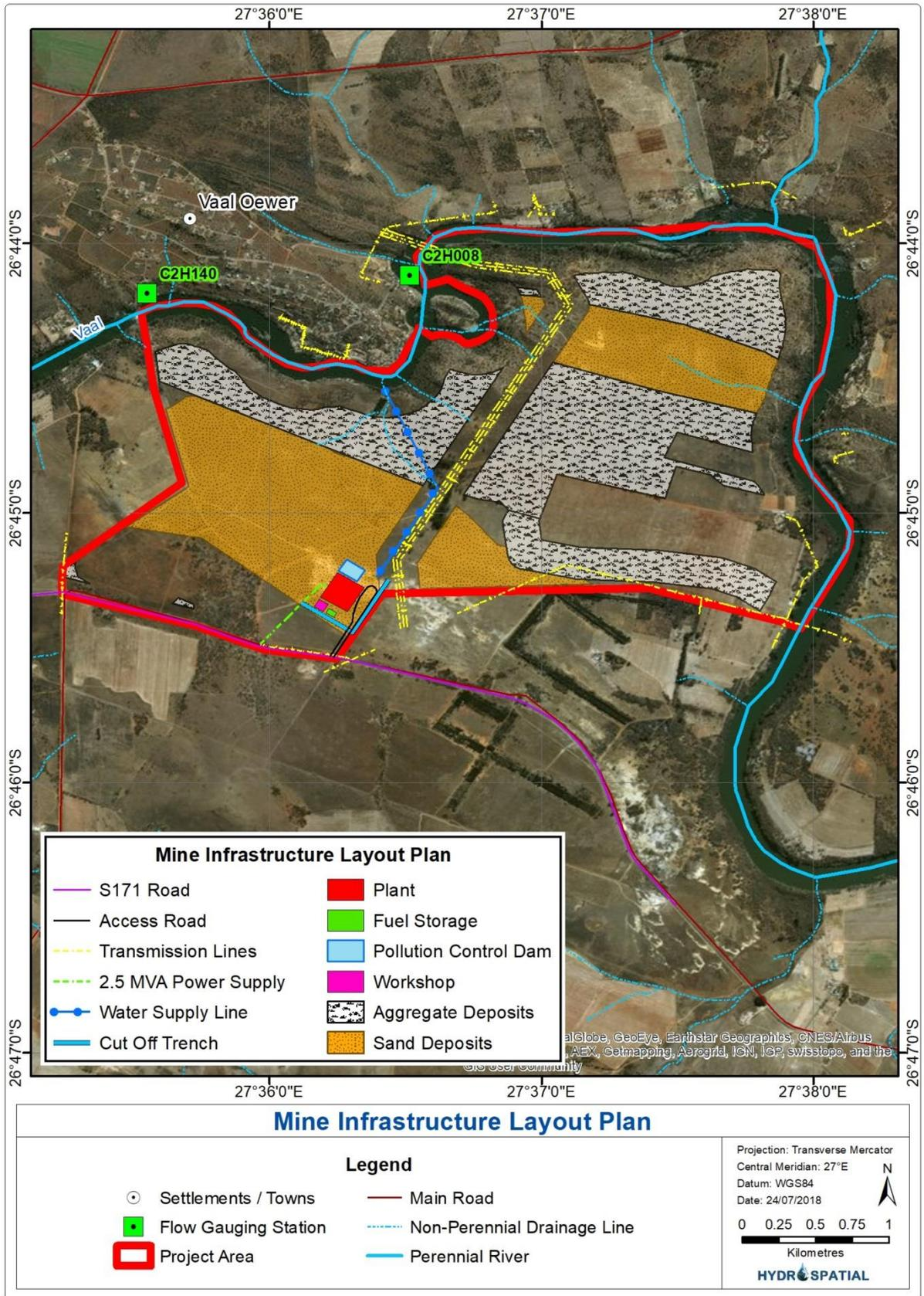
Figure 1-2: Mine infrastructure layout plan
