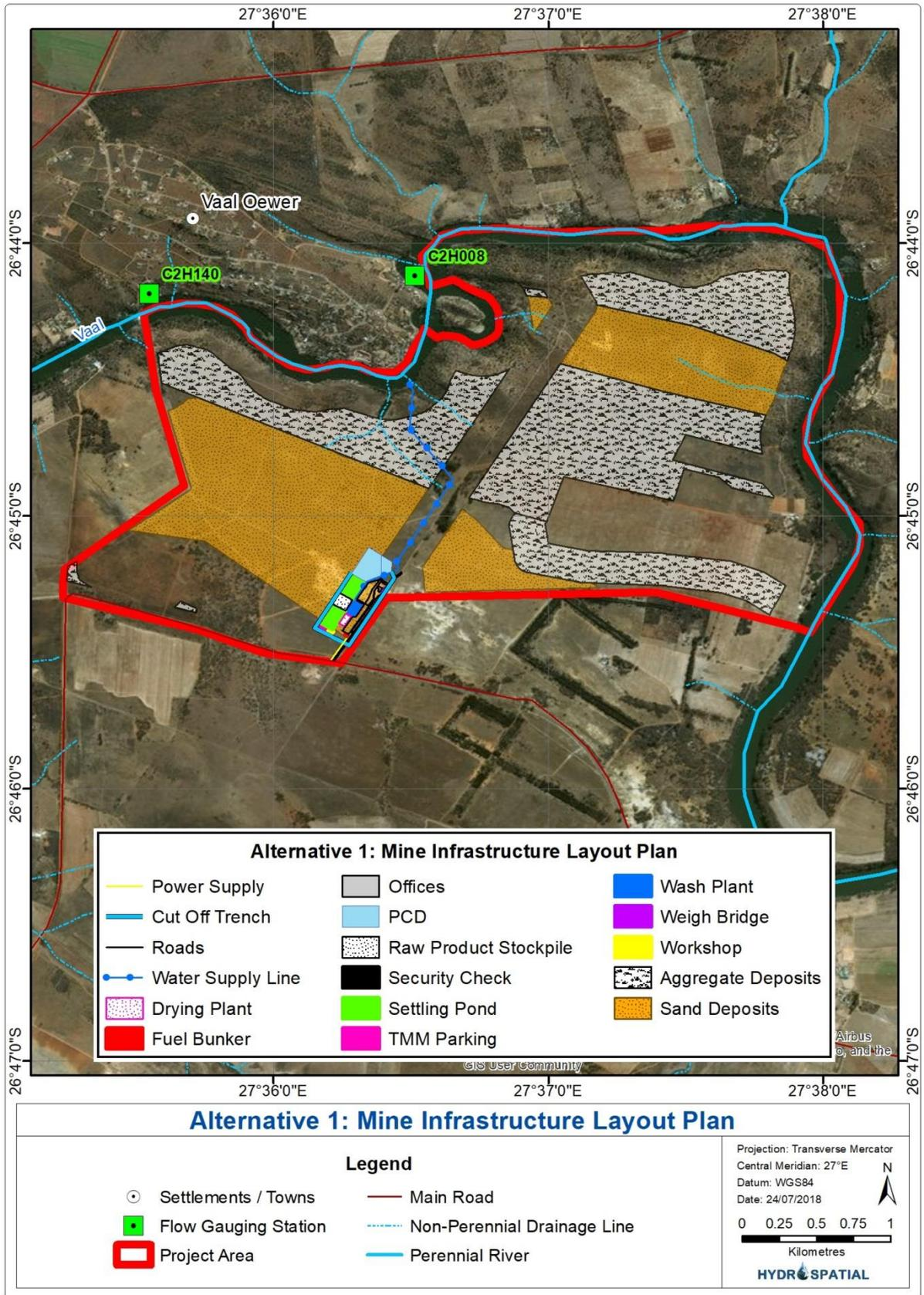
Figure 1-2: Alternative 1: mine infrastructure layout plan
