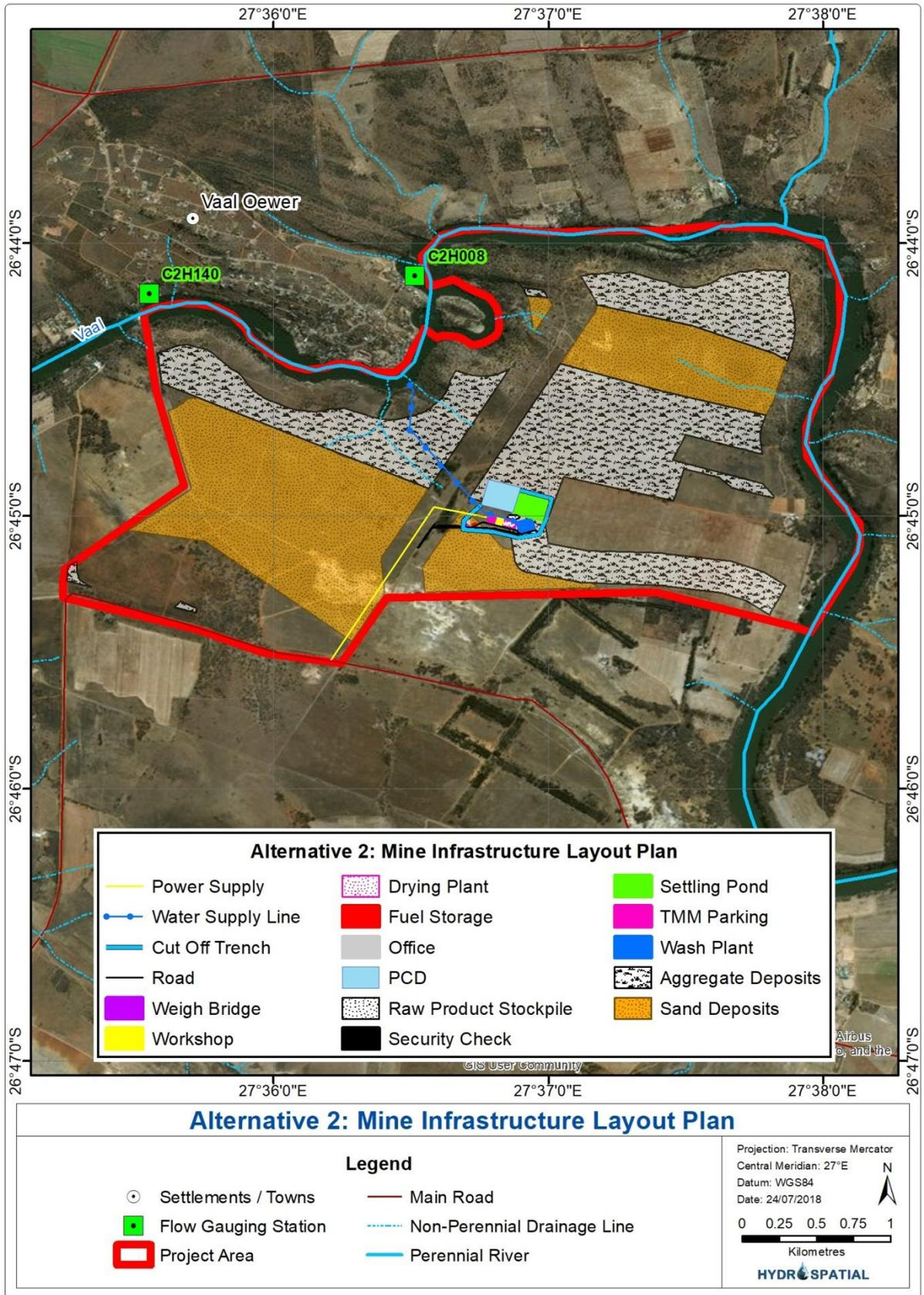
Figure 1-3: Alternative 2: mine infrastructure layout plan
