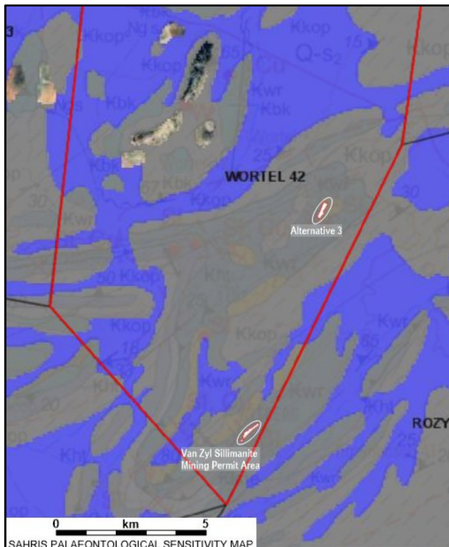
Figure 5. Palaeontological sensitivity of the Project Area. Grey – no palaeontological studies required. Blue - no palaeontological studies required, but a protocol for fossil finds is required. The clear patches in the north are unfossiliferous outcrops of the Gareskop intrusions.
