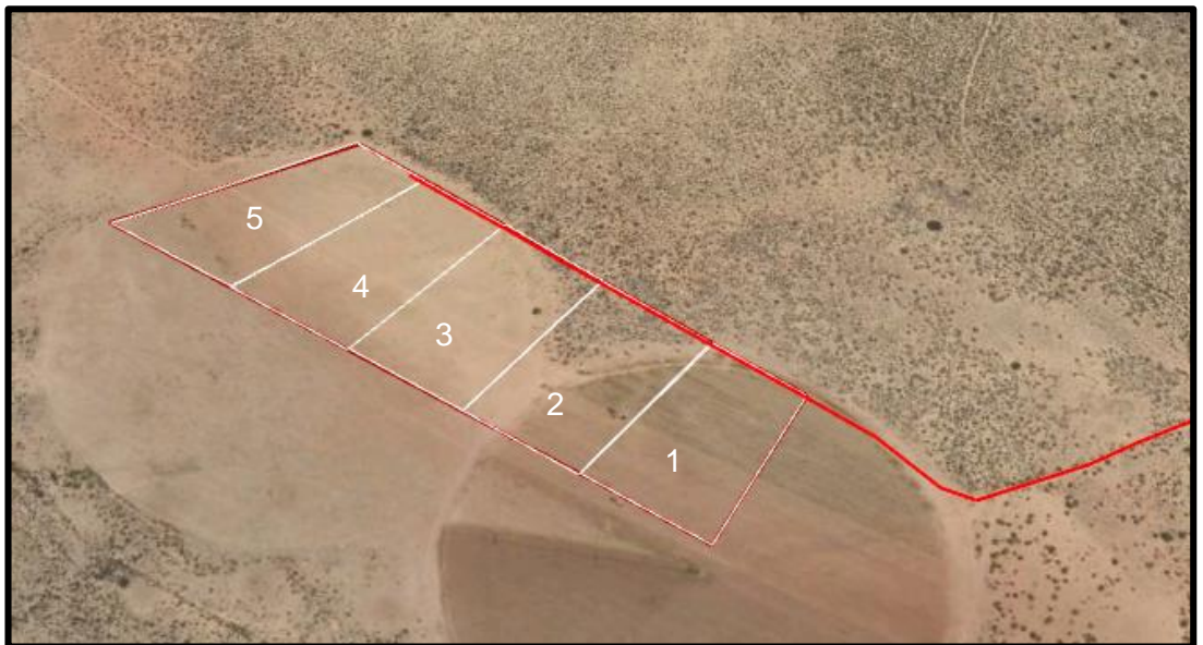
Figure 5: Proposed strip mining direction of the footprint area where the red line shows the existing access road.
