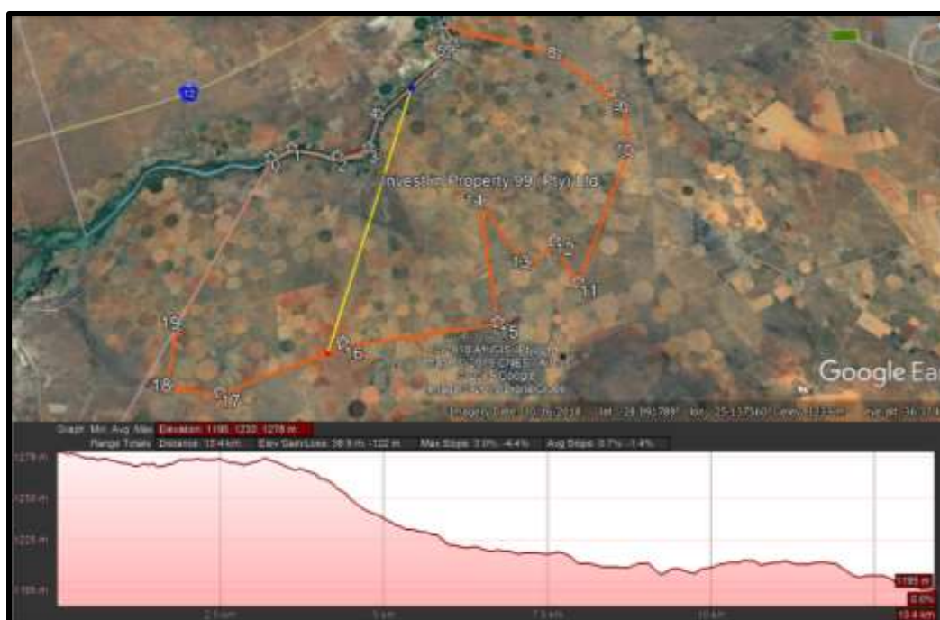
Figure 20: Elevation profile of the proposed mining area from the highest point in the south (1 278 mamsl) to the lower reaches of the Vaal River (1 195 mamsl).
