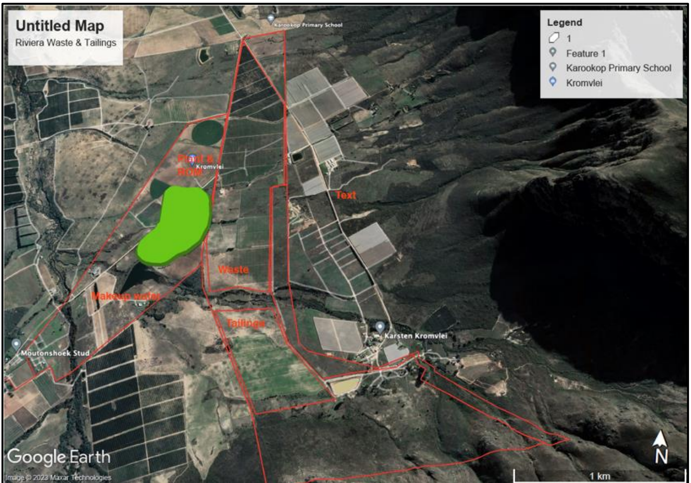
Figure 5: Satellite view of the proposed layout of the mining footprint, where the green polygon indicates the opencast excavation (School of Rock, 2023).
