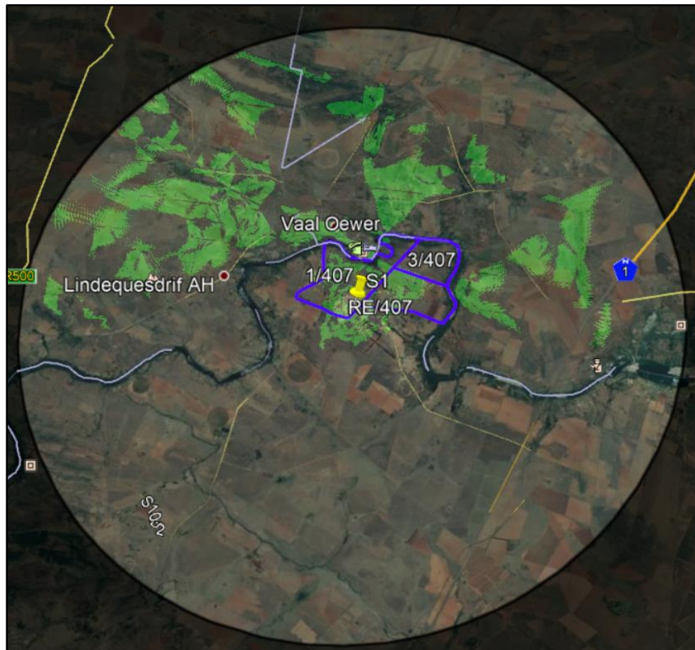
Figure 24: Viewshed analysis of S1) where the green shaded areas show the positions from where the operations will be visible (image obtained from Google Earth).
