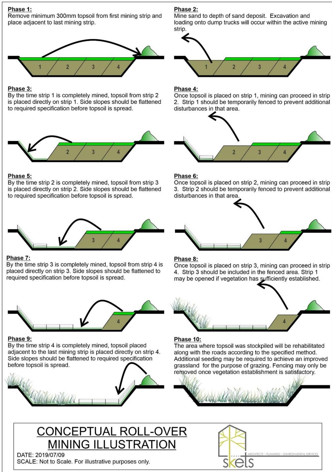
Figure 25: Conceptual roll over mining procedure (2)
