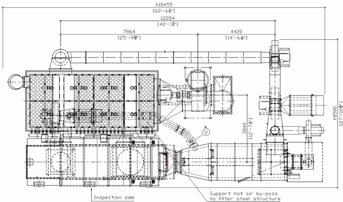
Figure 38: Plan view of a typical fluid bed sand drying unit
