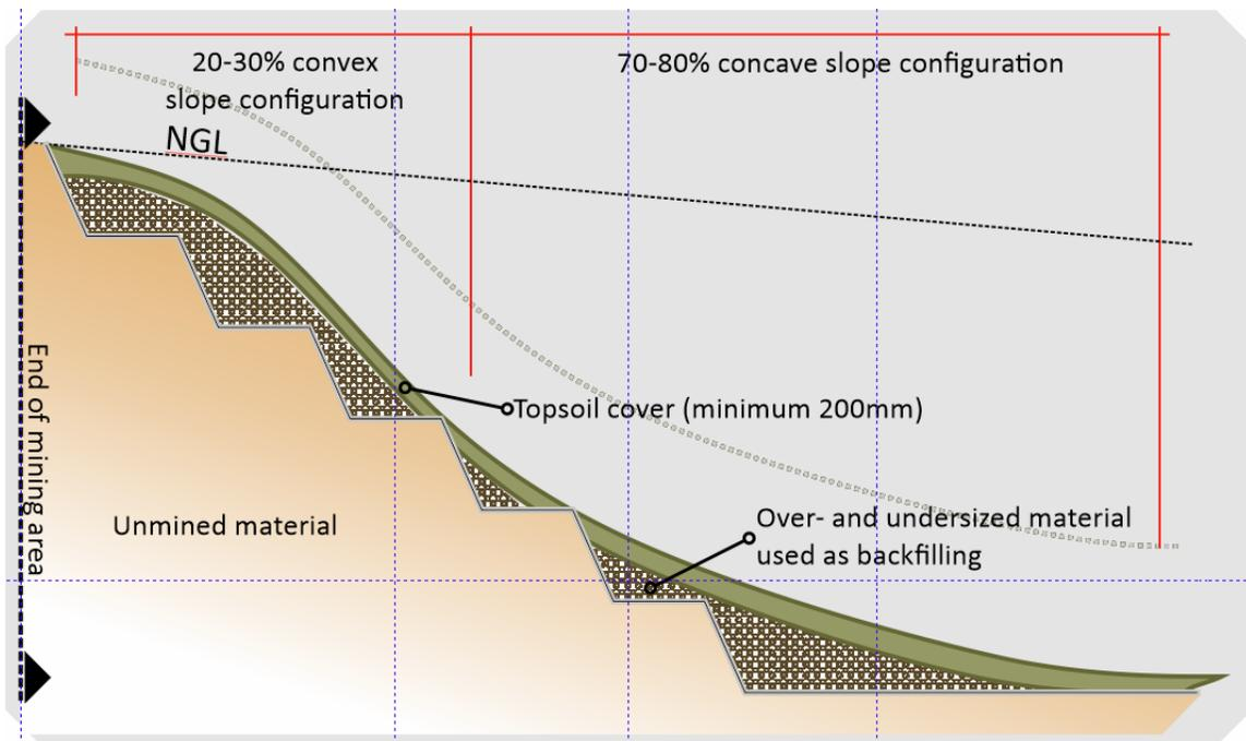
Figure 44: Ideal slope profile over benched face
