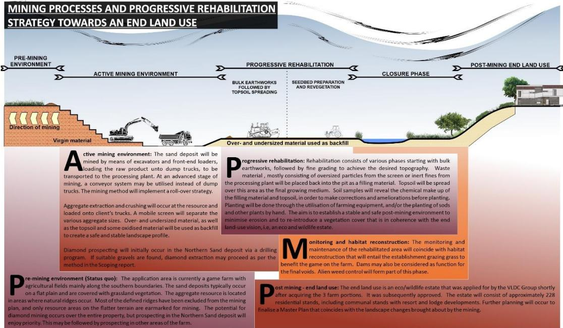
Figure 23: Mining processes and progressive rehabilitation strategy
