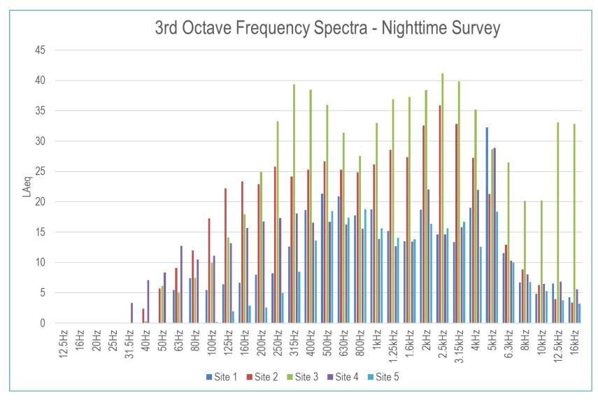
Figure 10: Nighttime Frequency Spectra
