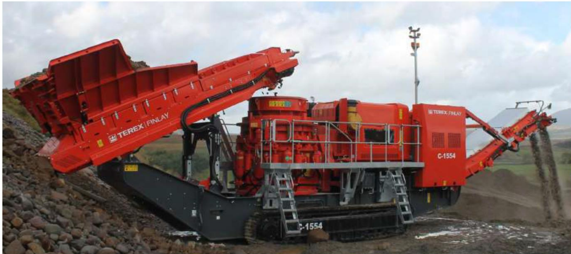
Figure 26: Example of mobile crusher
