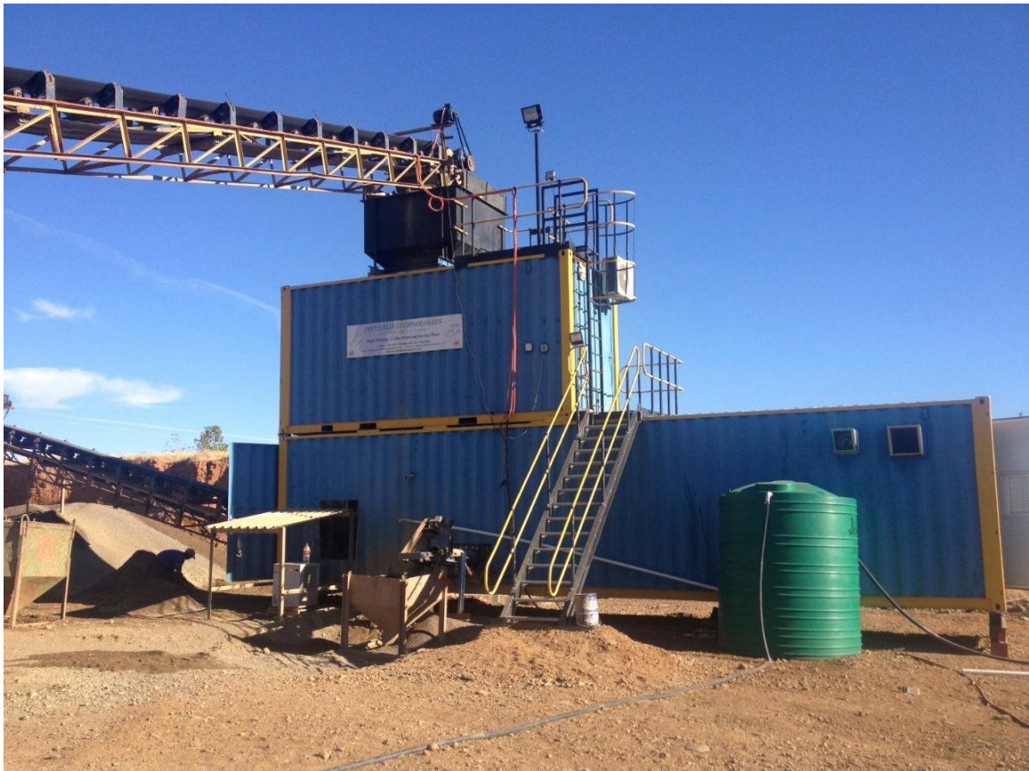
Figure 35: Typical setup of a diamond x-ray sorter
