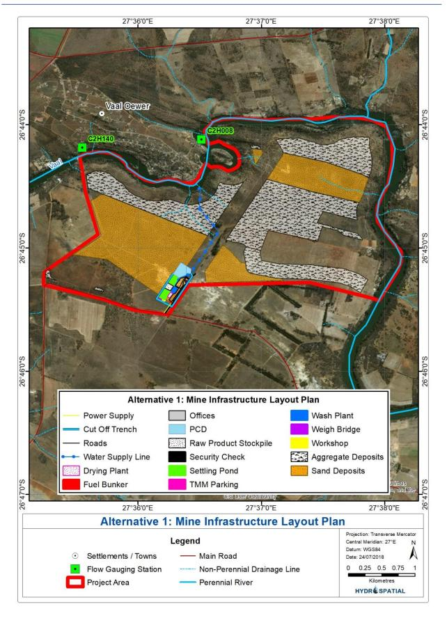
Figure 1-2: Alternative 1: mine infrastructure layout plan
