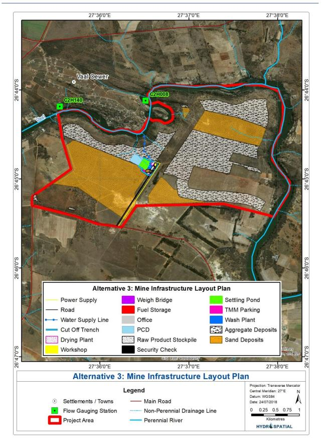
Figure 1-4: Alternative 3: mine infrastructure layout plan
