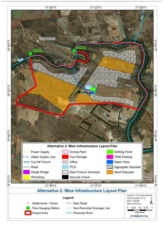
Figure 1-3: Alternative 2: mine infrastructure layout plan
