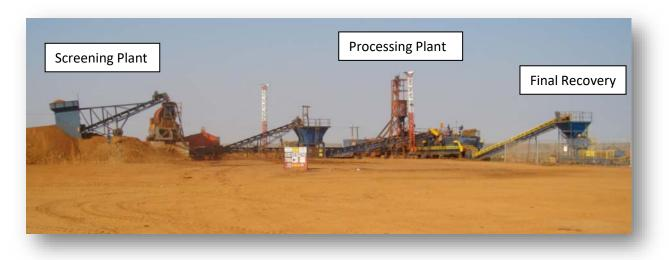
Figure 9 An example of the processing plant type proposed for the Woodlands bulk-sample
