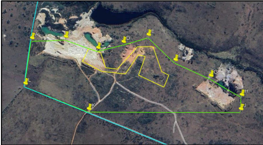
Figure 1: Satellite view showing the location of the proposed mining area (green polygon) in relation to the surrounding landscape where the yellow polygon indicates the Makana Brick mining permit area, and the blue lines show the boundary of Portion 3 of The Orchards No 233. (Image obtained from Google Earth)
