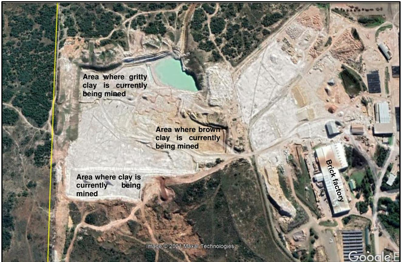
Figure 4: Satellite view showing the clay quarry in relation to the brick factory, where the yellow line shows the mining boundary (image obtained from Google Earth).
