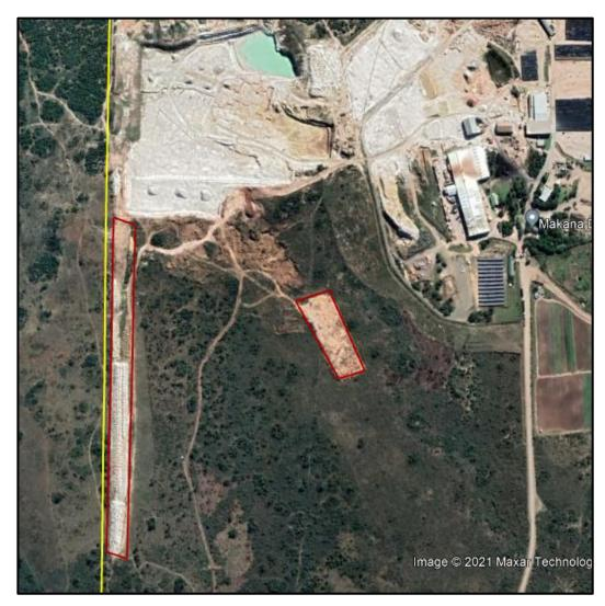
Figure 5: Satellite view showing the areas (brown polygons) currently used for the stockpiling of overburden from where the proposed aggregate products will be sourced (image obtained from Google Earth).
