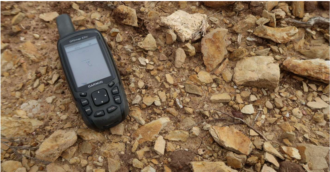
Figure 33: Semi degraded Lake Mentz subgroup siltstone exposed in a test pit at point 15 (Fig. 1).
