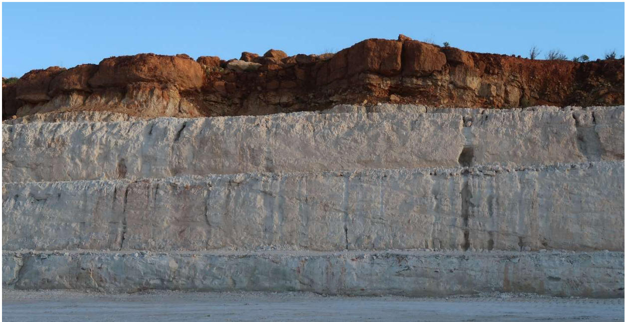
Figure 27: Kaolin derived from leaching of Waaiport Formation mudstones, and capped by silcrete crust in the south of the main brick clay quarry at point 12 (Fig. 1).
