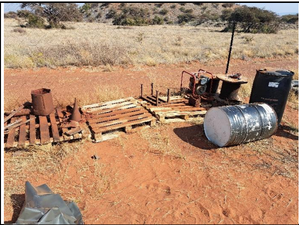
Drums that had to be removed to a bunded area
