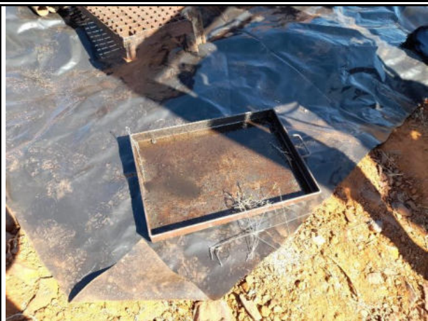
Drip tray used on site
