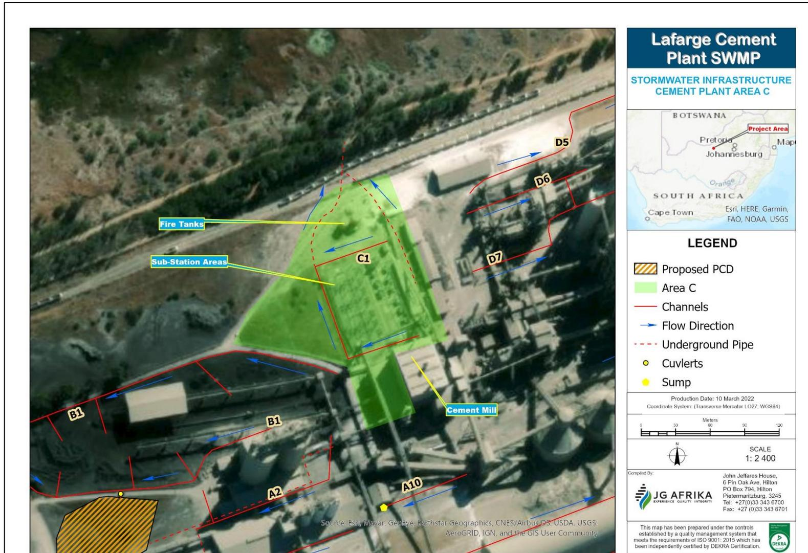
Figure 4-4 Lafarge Lichtenberg Cement Plant Stormwater Channels – Area C
