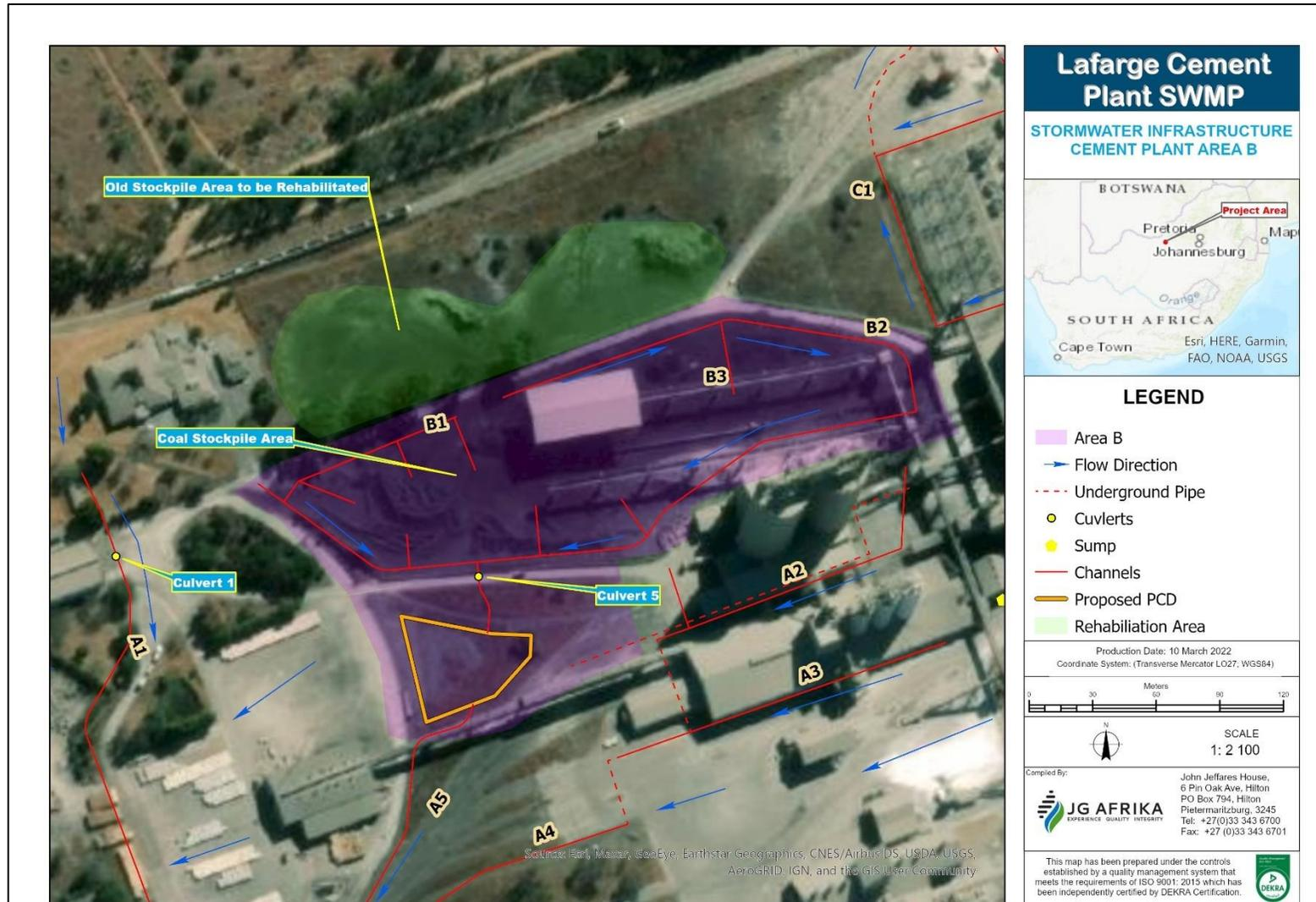
**Figure 4-3** Lafarge Lichtenberg Cement Plant – Coal Stockyard Area Stormwater Management – Area B
