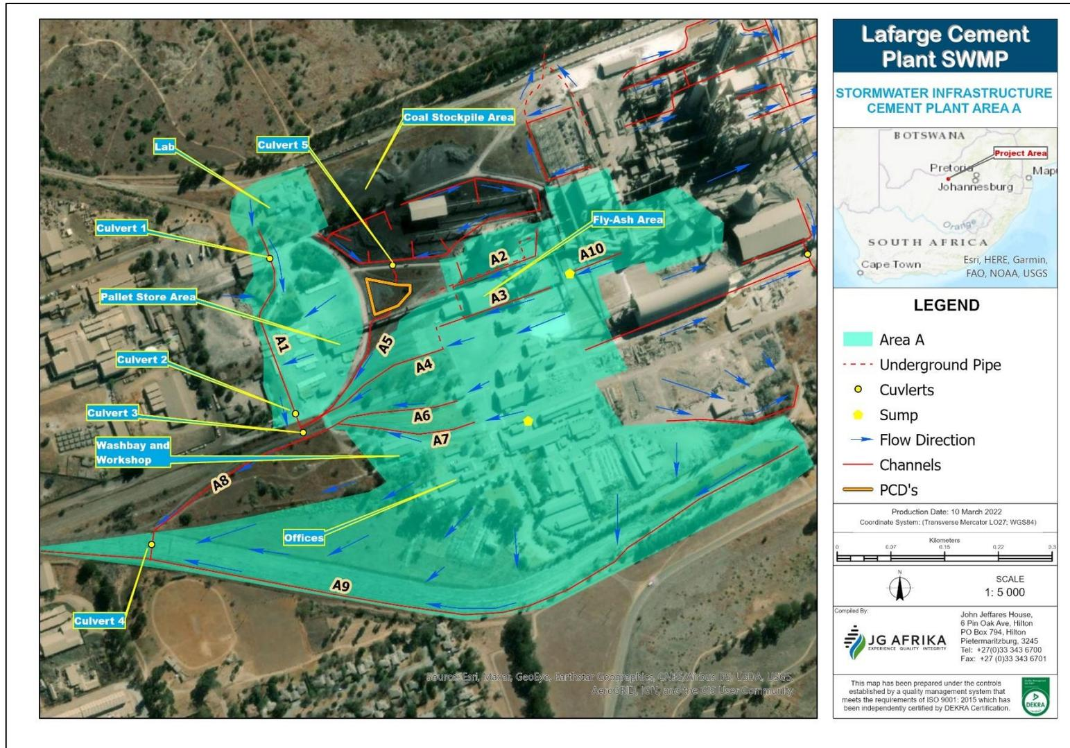
Figure 4-2 Lafarge Lichtenberg Cement Plant Stormwater Channels – Area A
