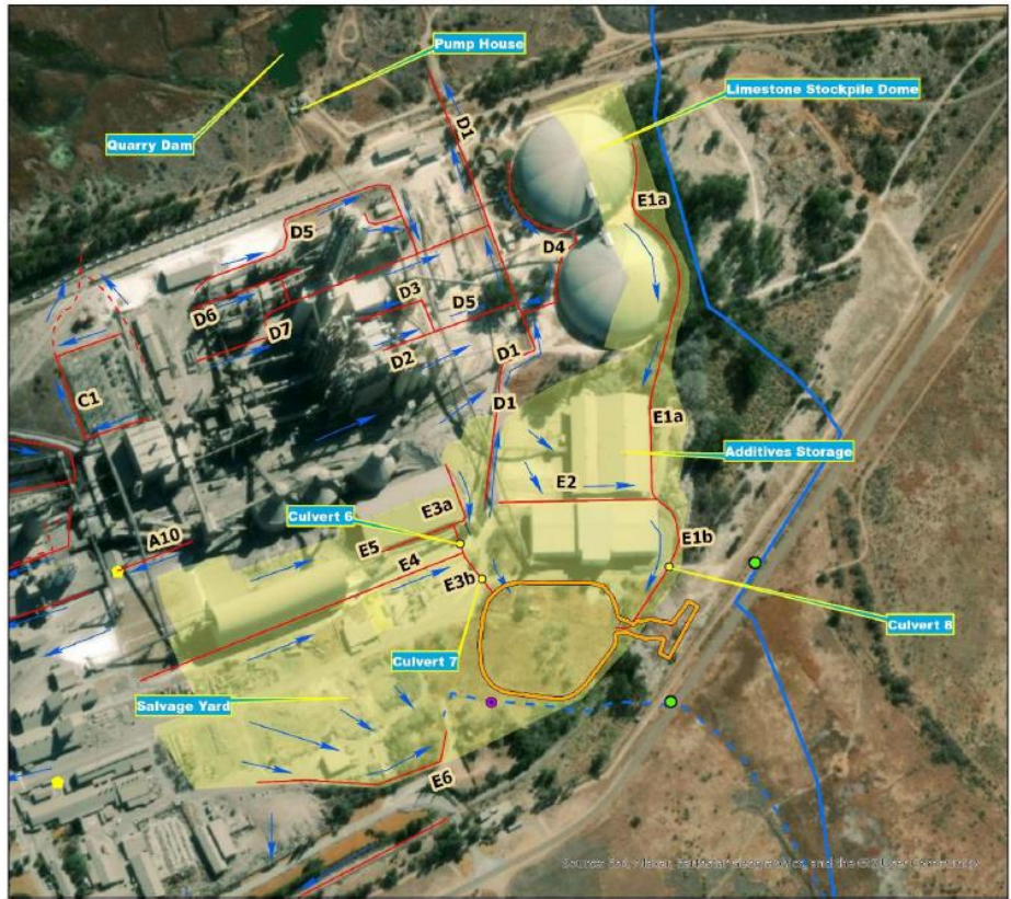
Figure 14: Lafarge Lichtenburg Cement Plant – Area E
