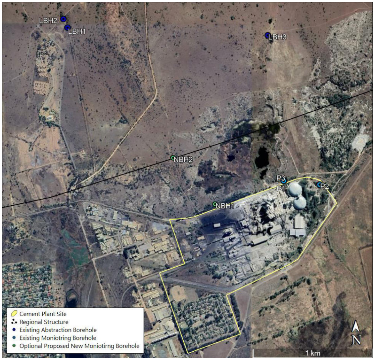
Figure 32: Cement Plant Groundwater Monitoring Network
