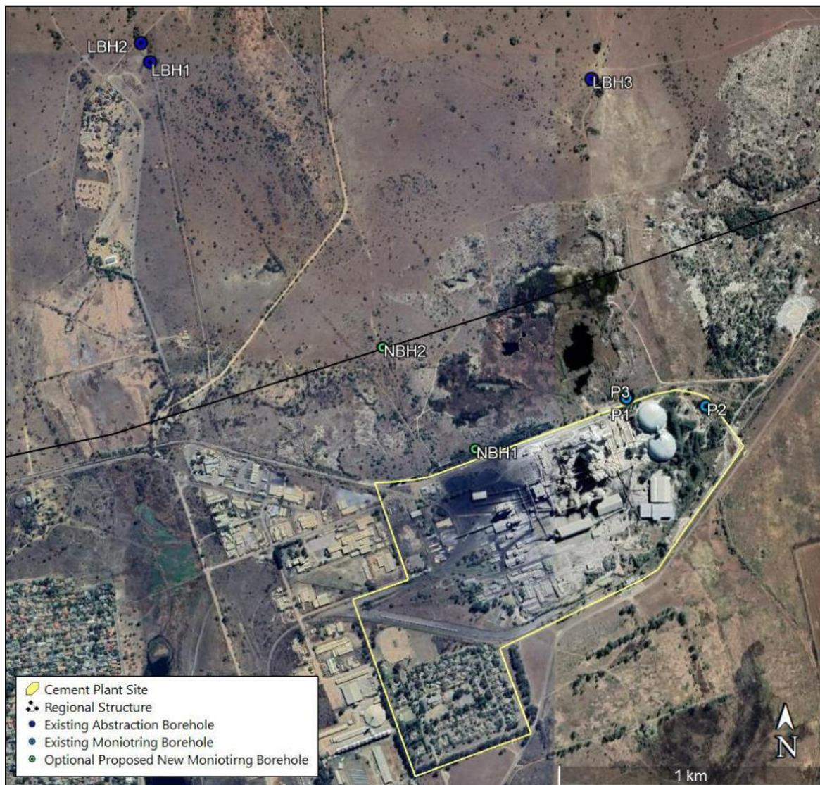
**Figure 20: Cement Plant Groundwater Monitoring Network**
