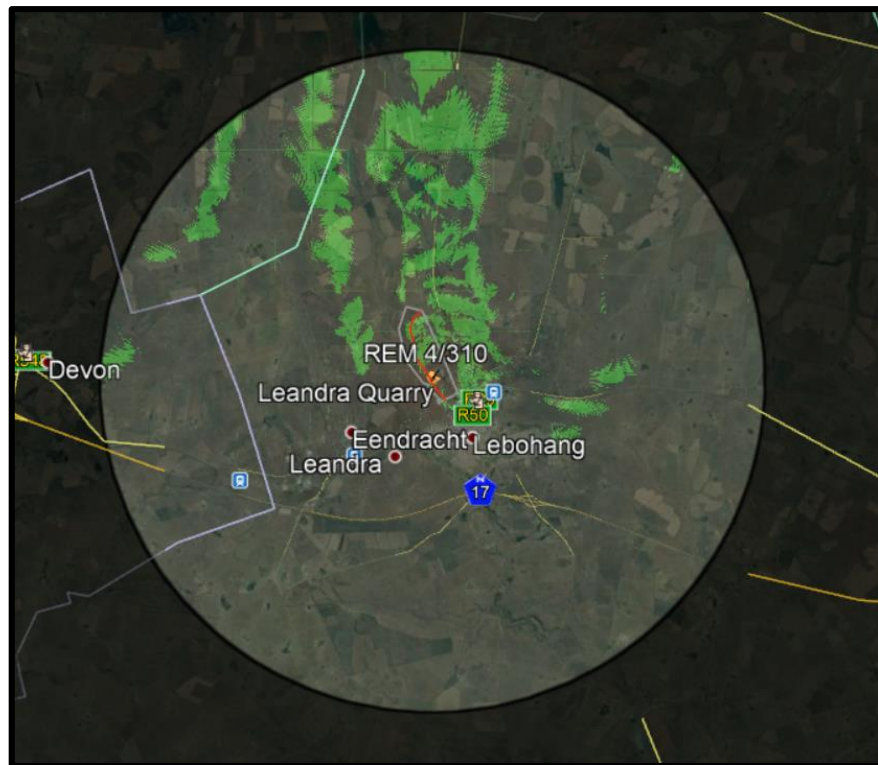
Figure 22: Viewshed of the proposed mining footprint where the green shaded areas shows the positions from where the mining area (Proposed mining area) will be visible. (Image obtained from Google Earth).
