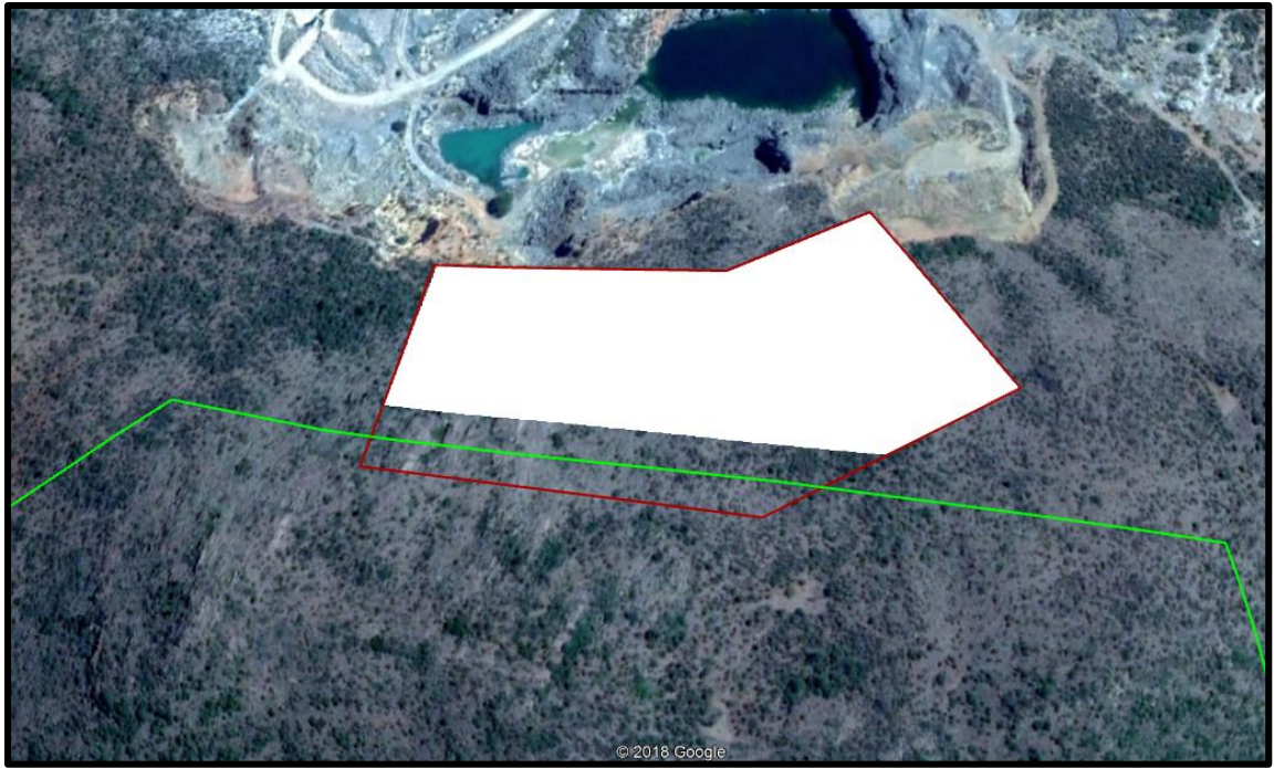
Figure 23: Satellite view of the proposed mining area (red polygon) in relation to the CBA 2 area (green line). The white shaded polygon represents the mineable area when the 20 m no-go buffer area is omitted.
