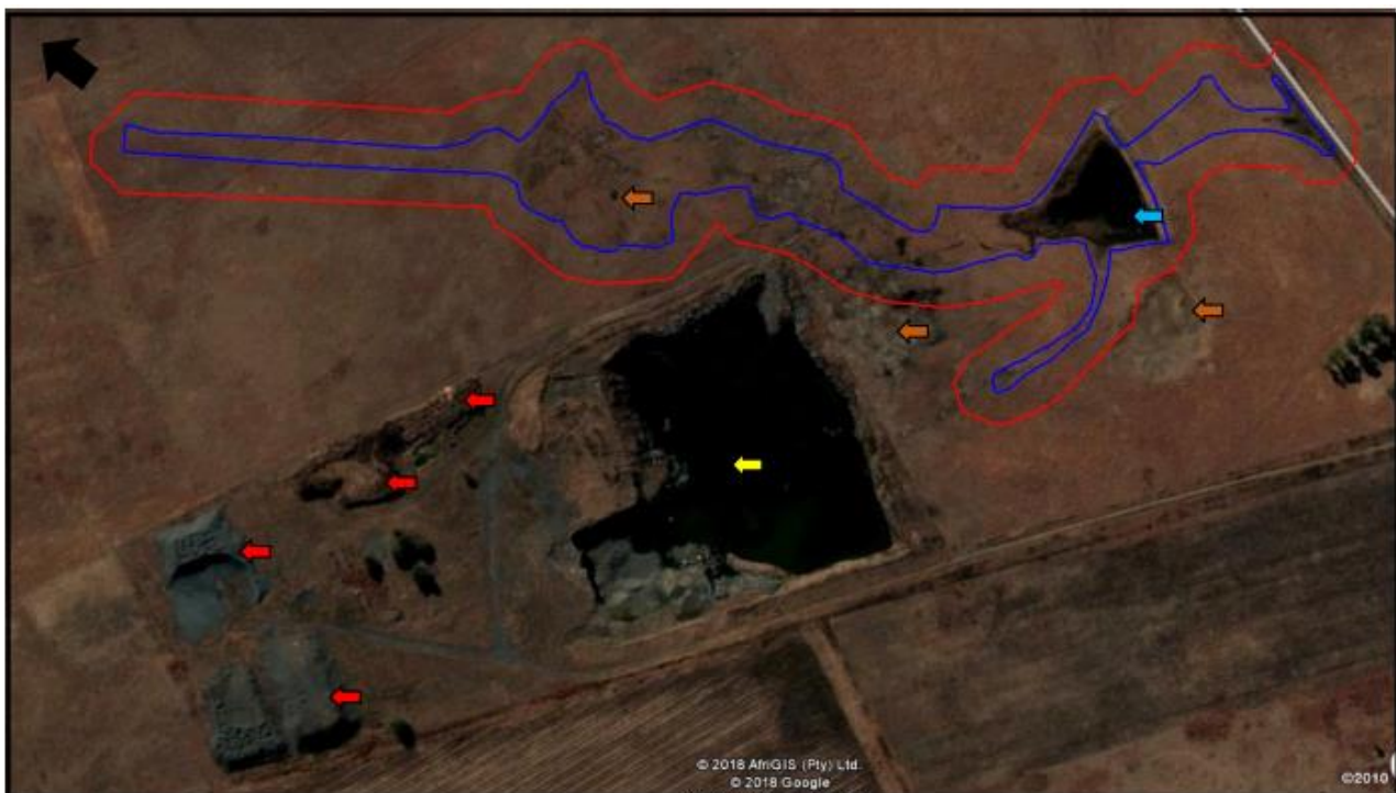
Figure 20: The blue lines indicate the unnamed watercourse and its 32m buffer (red line). The yellow arrow indicated the quarry filled with water. The orange arrows indicate the disturbed areas (mining permit areas), the red arrows indicate stockpiles of crushed material and spoil material and the blue arrow indicates the manmade farm dam.
