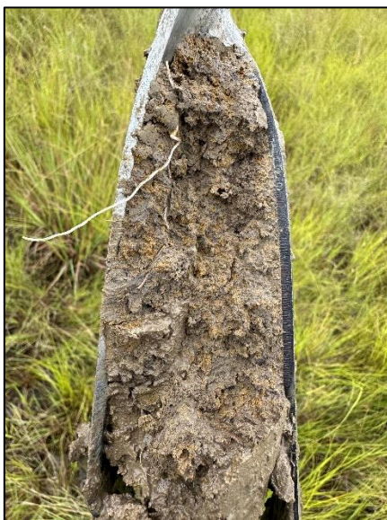
Photo 3: Example of a typical seasonal saturated soil (grey matrix with abundant soil mottles).
