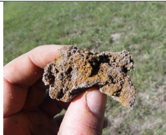
Photo 17: Mottles (accumulation of iron and manganese oxides) within the soft plinthic B horizon. Grey colour is the result of gleying.
