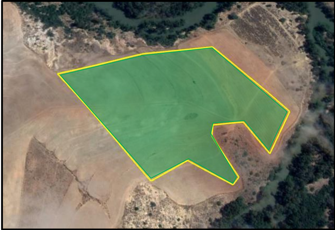
Figure 6: Satellite image (2019) of the proposed mining area to be rehabilitated upon final closure of the Drieheuvels Quarry. The green polygon shows the excavation area to be sloped and returned to agricultural use after rehabilitation.
