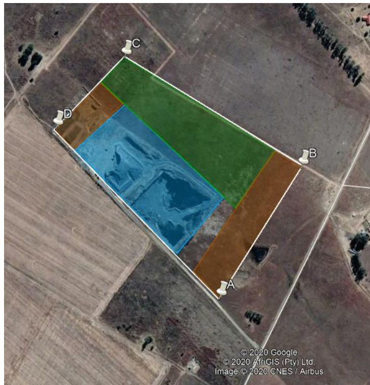
Figure 1: Satellite view of the proposed mining area (white outline), where the blue shaded polygon indicate the proposed opencast area ( \pm 8.7 ha), the brown shaded polygon shows the proposed overburden and stockpile areas ( \pm 6.6 ha), and the green shaded area represents the proposed general surface to be altered ( \pm 8.7 ha). (Image obtained from Google Earth).
