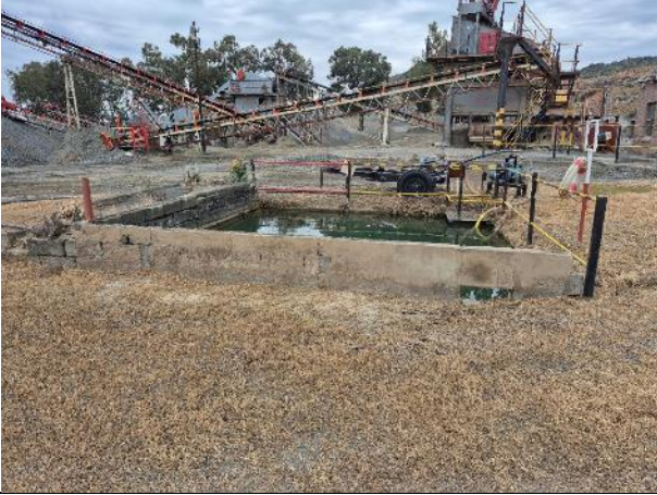
Pit to be supplied with a mesh grid to prevent injuries
