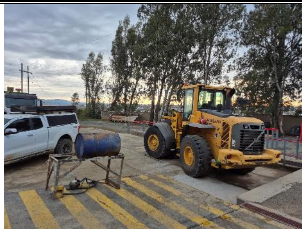
Building removed to increase service bay area. Also note drum used to contain contaminated water that collects in drip trays.
