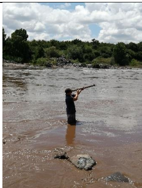
Photograph 15: Determining turbidity with a clarity tube.
