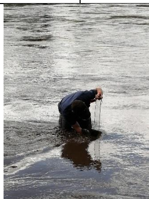
Photograph 17: Determining flow velocity with a flow velocity rod
