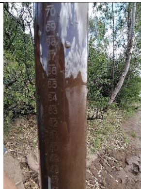
Photograph 16: Clarity tube indicating high level of turbidity and total suspended solids.
